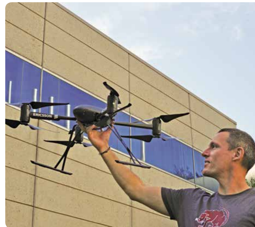
Autonomous platforms, such as this unmanned aerial vehicle (donated to CSIRO by Ericsson Australia), provide cost-effective surveillance systems for our borders.
